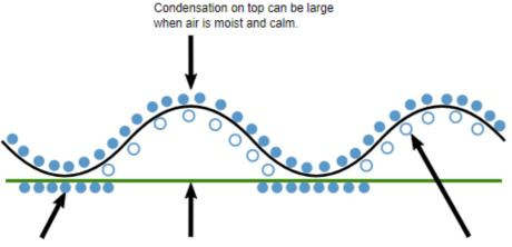
Paper in contact with cladding, gets cold: condensation occurs and gets absorbed by paper. Can be significant if attic air is moist.
